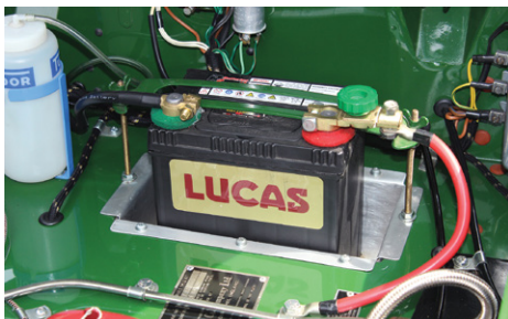
Battery located under bonnet for access.
