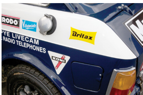
Original and new positions for fuel cap.
