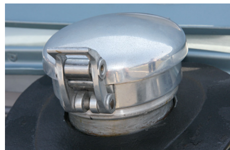
Quick-release fuel cap for fast refueling.
