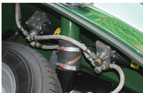
Twin fuel pumps for reliability in the race.
