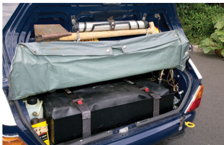
Rubber fuel tank and tools inside boot.
