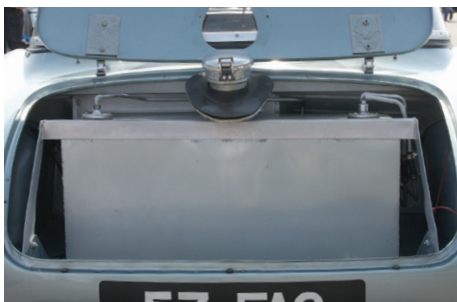
Huge fuel tank filled the boot.
