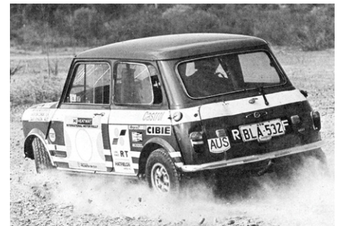
Photo from SCW shows Aus body with Mk1 taillights, UK plate, MGB reversing lights, upswept exhaust and crease in bootlid.
