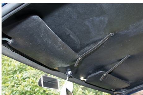
Straps prevent visors falling on dirt roads.
