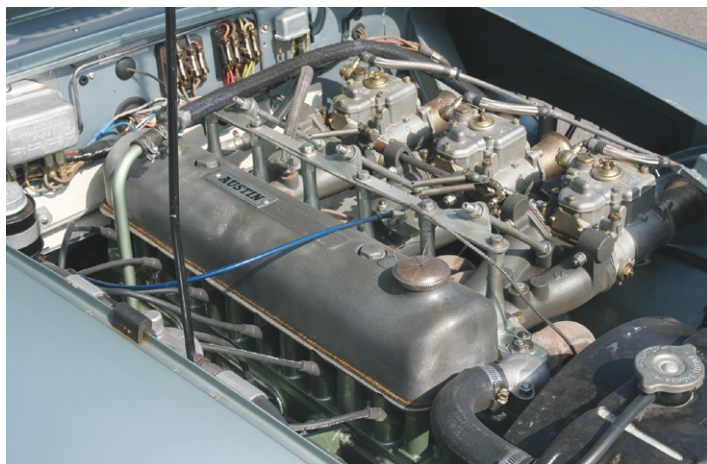
Weslake alloy cylinder head and triple Weber carbs helped push the 1963 cars into the Prototype GT class for Sebring.
