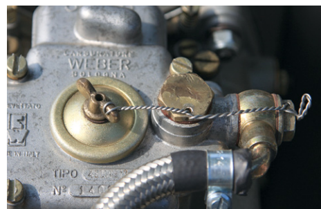
Important bolts were wired in place.
